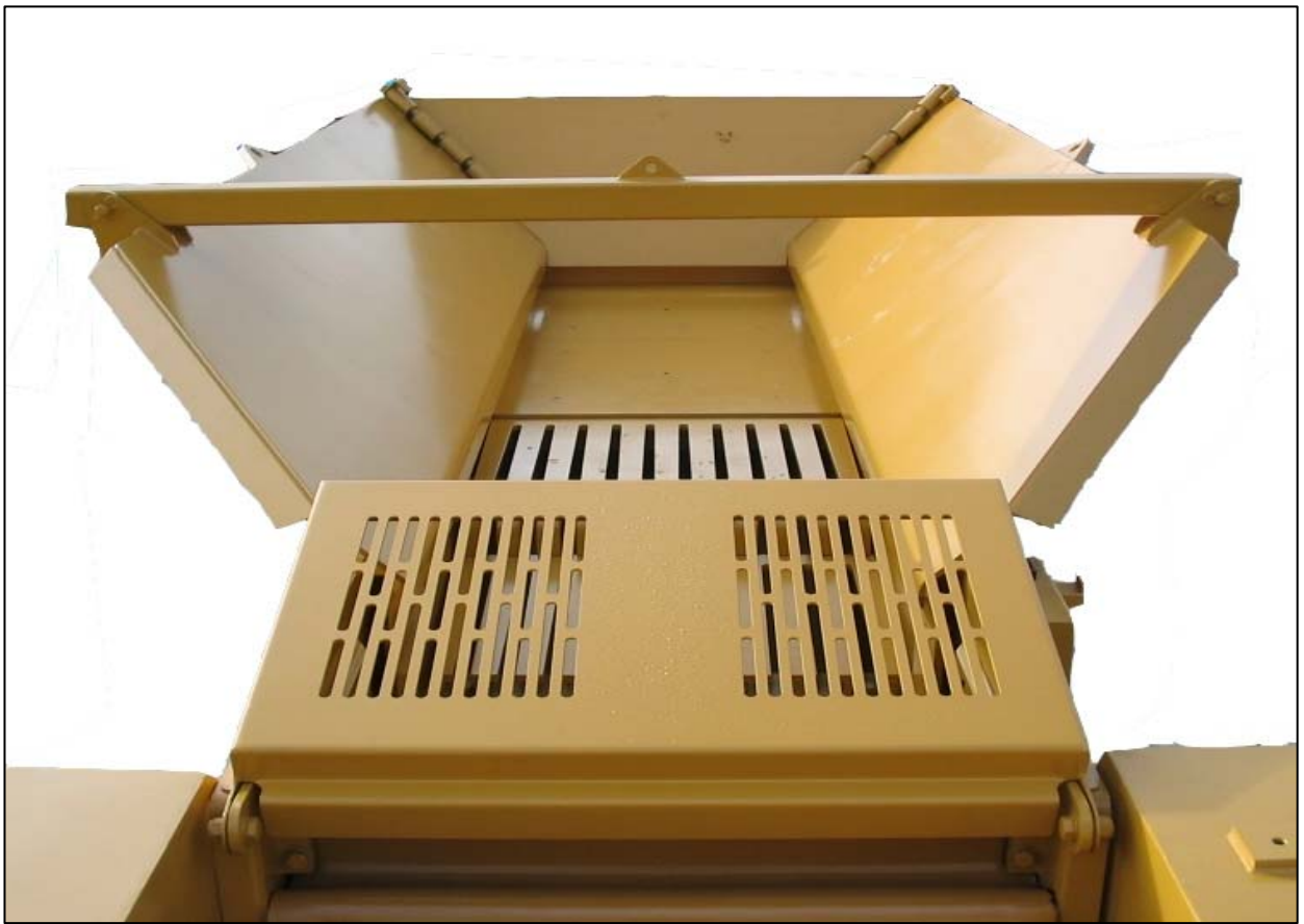
Large vibrating feeder with grizzly and discharge conveyor for fines.
