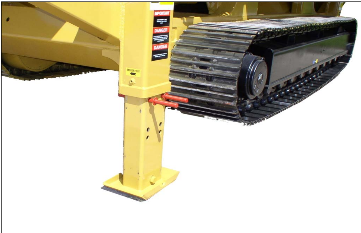
Machine raises on its hydraulic legs to facilitate cleaning and servicing of tracks
