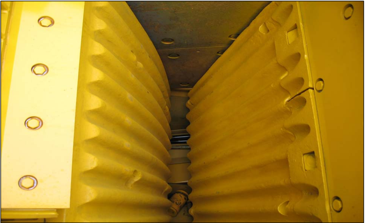
Powerful Jaws able to crush even the toughest rock products
