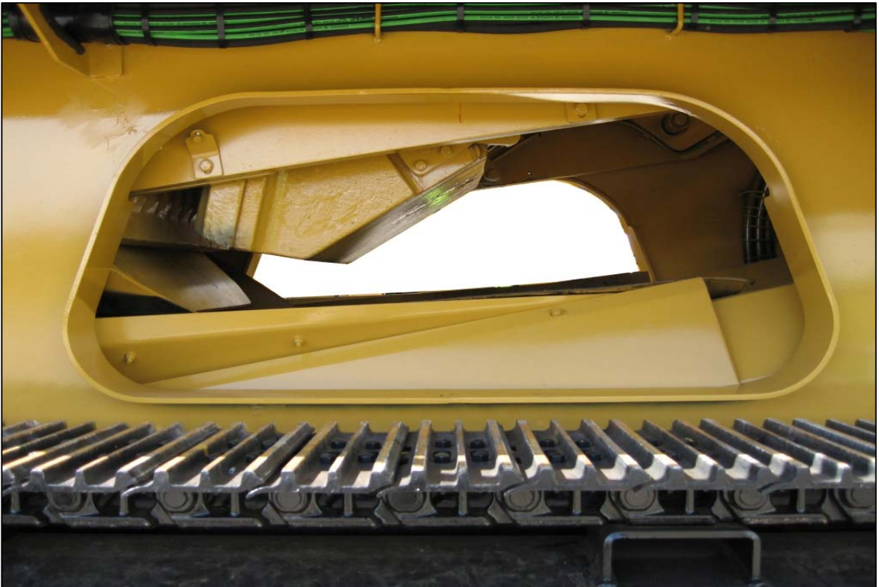
Large gap between discharge point of crusher and conveyor eliminates blockages and facilitates cleaning.
