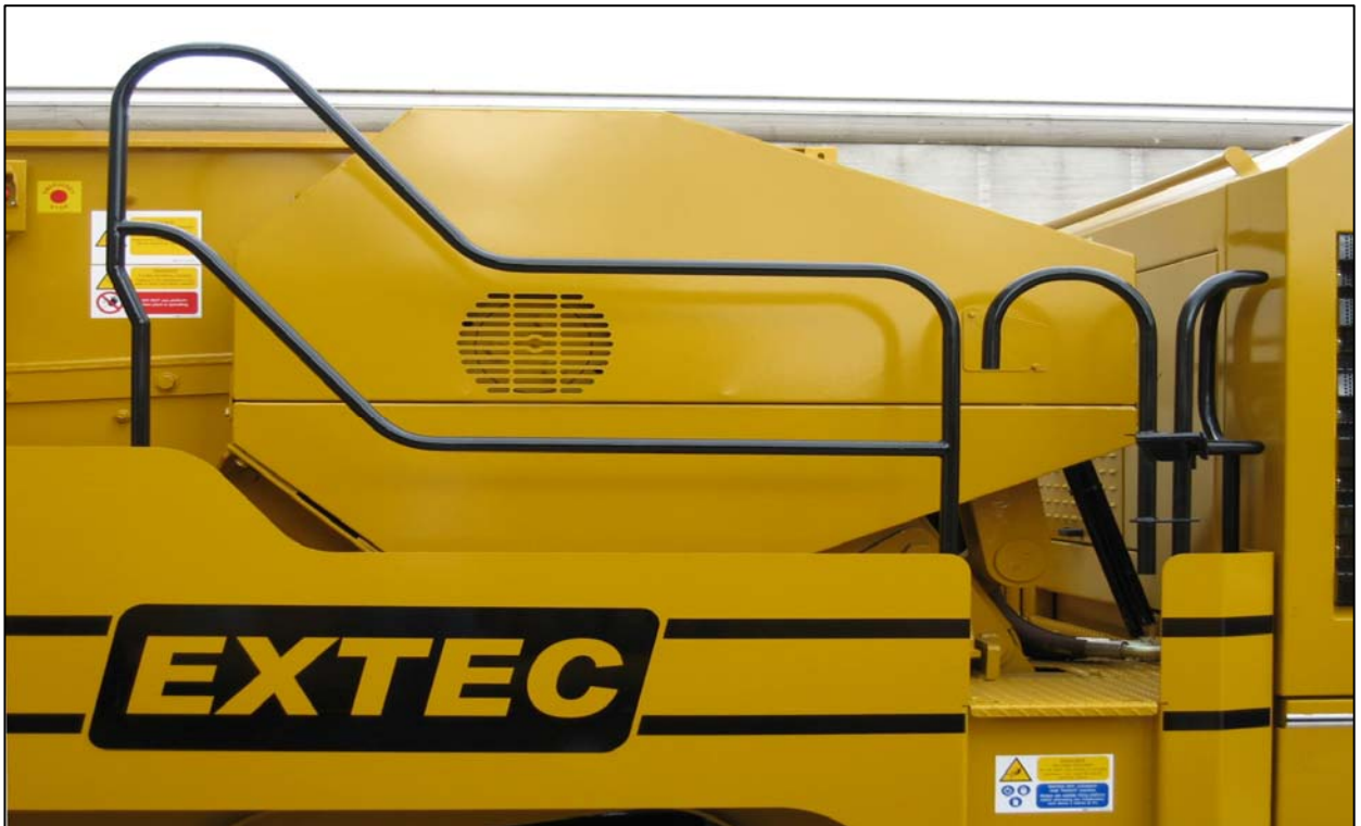
Maintenance platforms are provided on the right hand side of the crusher
