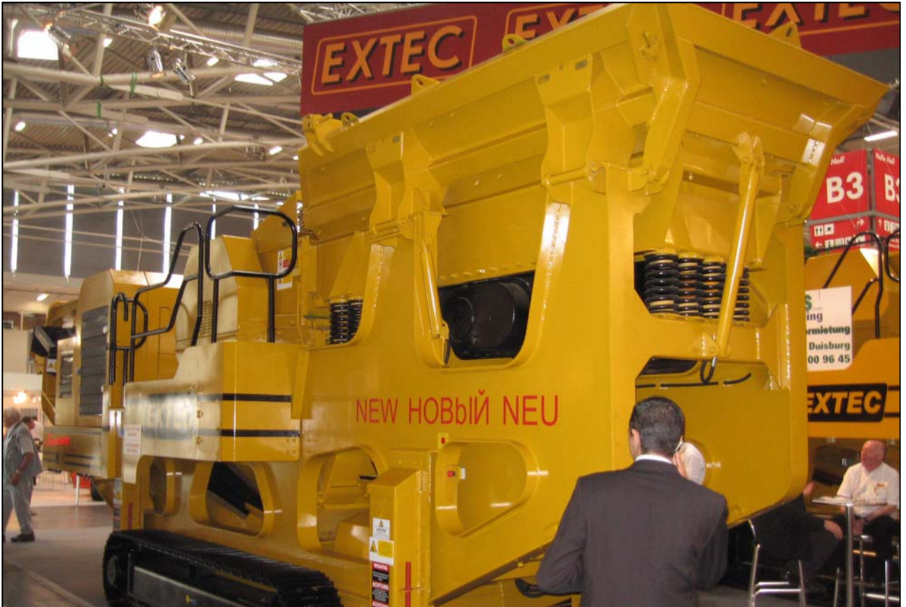
Heavy Steel Web and Flange Chassis
