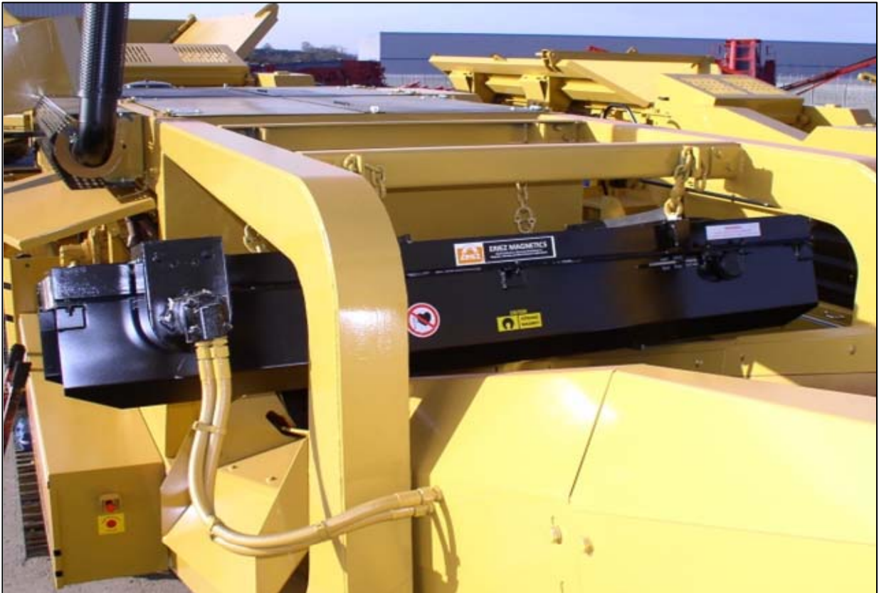
Magnetic Separator – effective removal of metal
